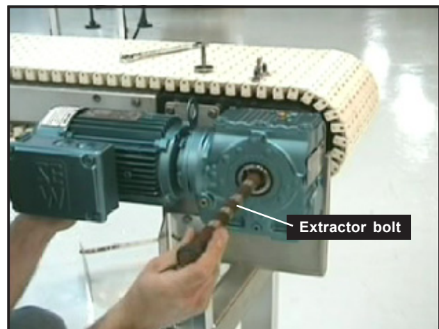
Figure 43: Insert extractor bolt to drive gearbox off shaft
