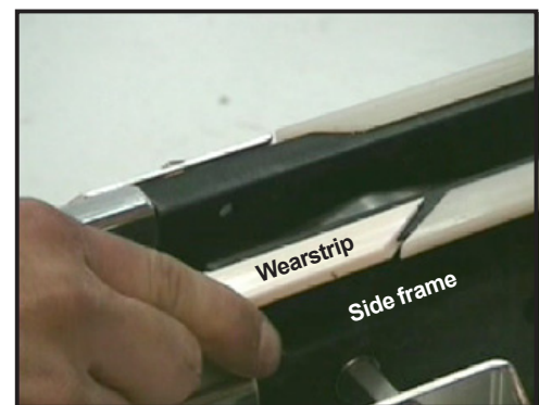
Figure 14: Slide wearstrip into side frame
