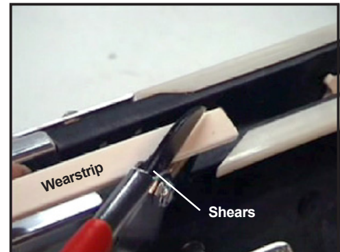
Figure 13: Cut wearstrip at 60° angle
