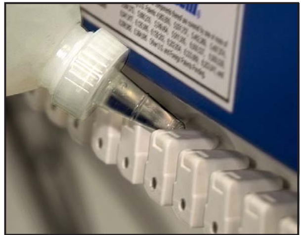
Lubricate the conveyor wearstrip with silicone oil
